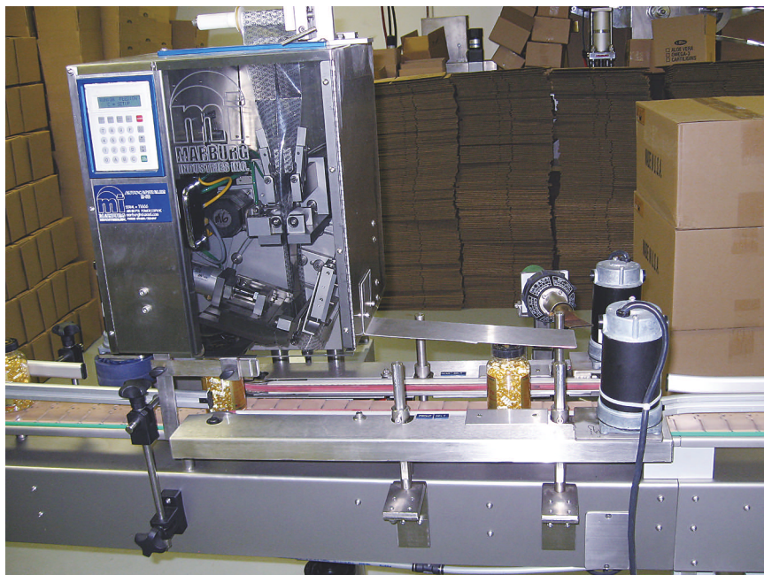
Labels are applied by a wraparound labeler, left, that is equipped with a hot-stamp printer that prints a lot number and production and expiration dates onto the label before it is applied. A continuous-motion neck bander, above, cuts tamper-evident bands from a tube of material and places them over the tops of the bottles.
