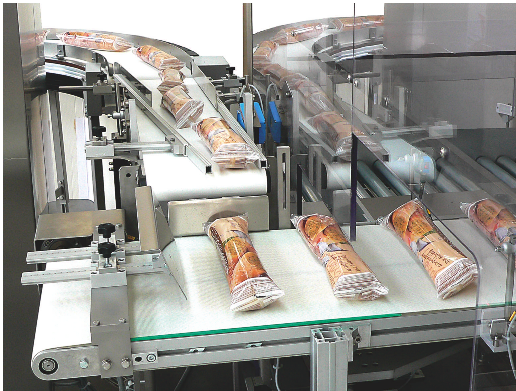
The robotic packaging system, left, must handle a variety of packages because customers work with different case sizes and different packing configurations. The cases can have from three to six layers, with three to nine baguettes packaged in each layer. The baguettes are arranged transversely on the discharge belt, above, to increase packaging reliability and reduce line speed.
